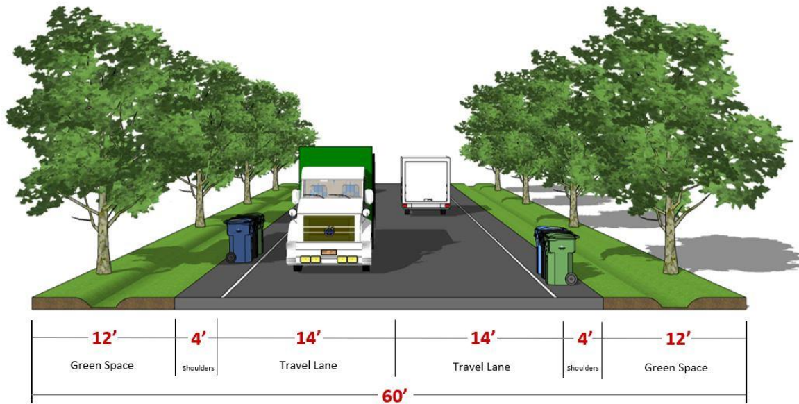
Figure 60: Recommended Section - Local (Rural)
